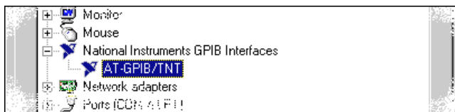
Figure 2-13. GPIB Interface That Is Working Properly
